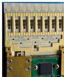
Radiator Elements GaAs SOC Chip (LTCC) Power divider (LTCC) Beam Controller
